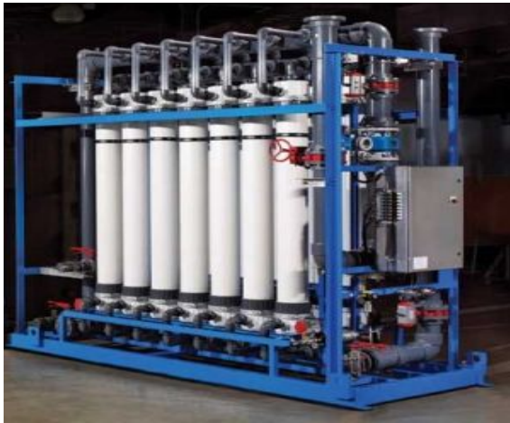
Skid Mounted UF Plant
